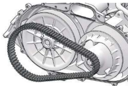
4. with the kit-out pin for driven pulley (special tool) against the driven wheel as shown in the figure of the hole, make the driven wheel open.
